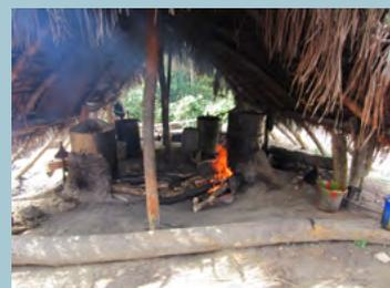
The distillation area with fire for heating up the fermented juice. Notice the firewood burning
